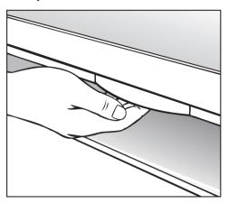
■ Press the release catch inside the door grip.
